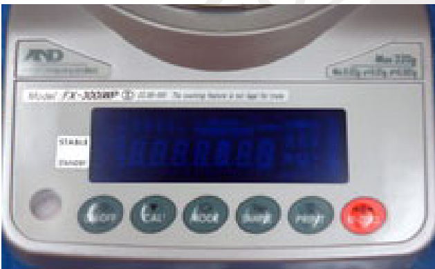
Function Buttons – on/off, cal, mode, sample, print and zero
